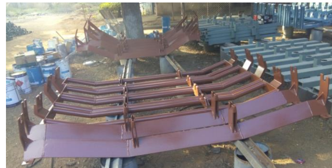
Standard idler base frames – Mass production on ROBOTIC Welding Machines
