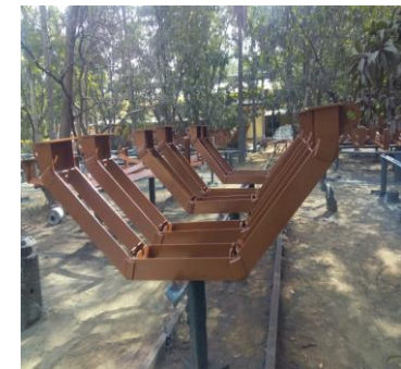
Standard idler base frames – Mass production on ROBOTIC Welding Machines
