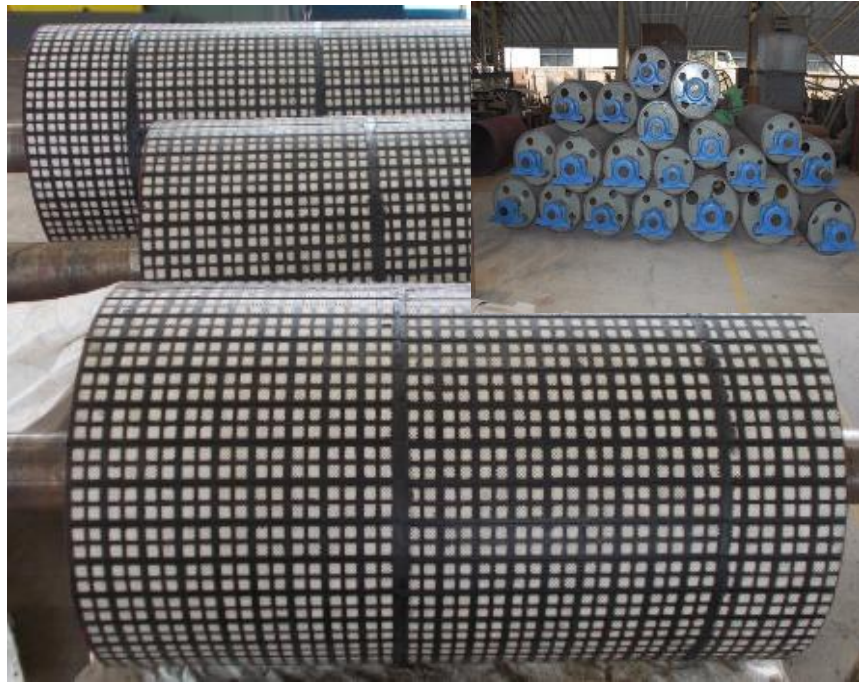
Pulley lagged with Ceramic Tiles
